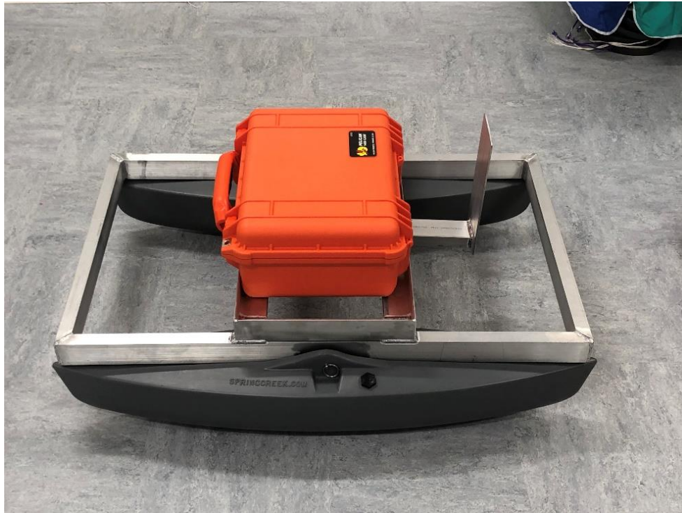
Figure 2-1. Pontoons, Pelican case, and aluminum frame.
