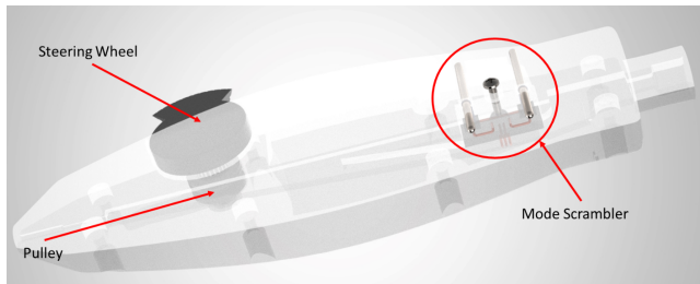
FIGURE 5 A computer rendering of the handle designed for this falloposcope. The outer material has been made partially transparent, so the internal mechanical assemblies are visible. This displays the interaction of the pulley and steering wheel as well as the assembly of the mode scrambler.
