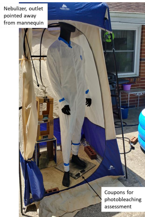
Figure 7. Exposure booth showing mannequin and nebulizer placement.
