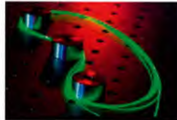
Figure 38: Twisted fibre on a kidney-shaped spool for improved pump absorption.
