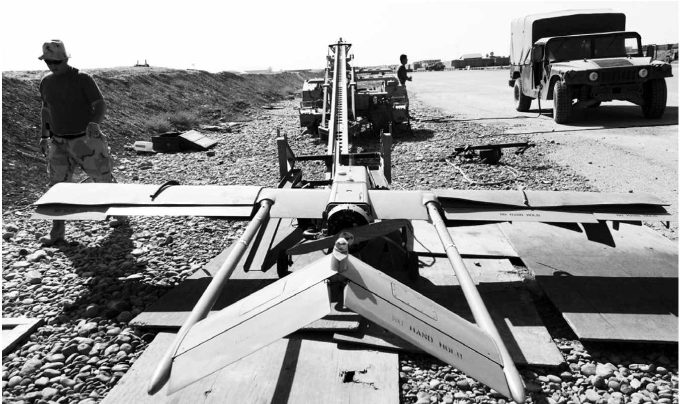
Tennessee Army National Guard Sgt. Ken Kay, 278th Armored Cavalry Regiment, prepares to launch a RQ-7 Shadow 200 Tactical Unmanned Air Vehicle for a mission at Forward Operating Base Warhorse, Iraq, on 28 May 2005, during Operation Iraqi Freedom. (Photo by SSgt. Suzanne M. Day, USAF)
