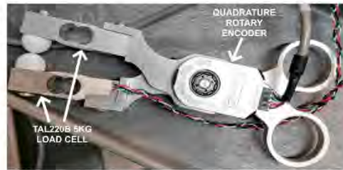
FIGURE 1: Grasper device hardware including load cells on jaw ends, hemispherical attachments near jaw tips, and encoder attached to metal body
