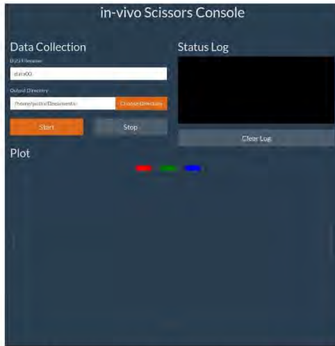
FIGURE 2: Graphical user interface used during data acquisition for file selection, titling, and providing live feedback of load cell and encoder readings
