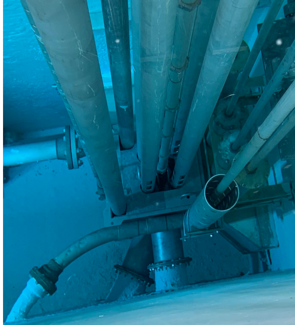
Figure 16. Overhead view of Ohio State University nuclear reactor. The curved tube is the pneumatic "rabbit tube" facility used in this study.
