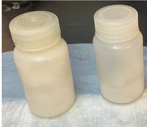
Figure 17. Containers used to transport sample groups through rabbit tube for irradiation.
