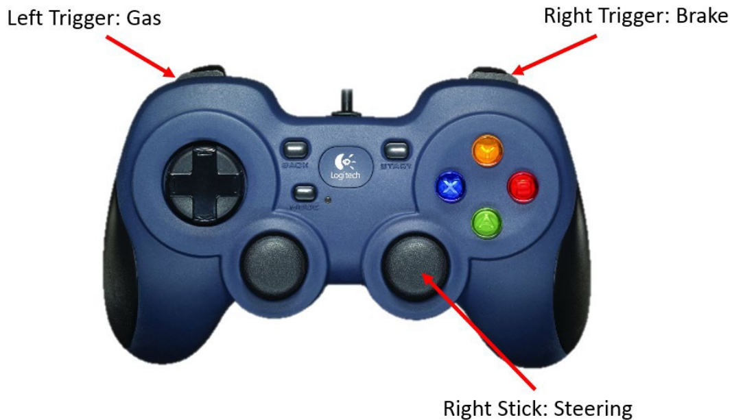
Fig. 2 Controller layout for robotic mobility operator's controls
