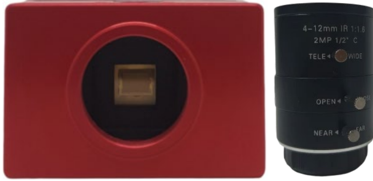
Fig. 3 DAVIS346 and 4–12-mm telescopic C-mount lens
