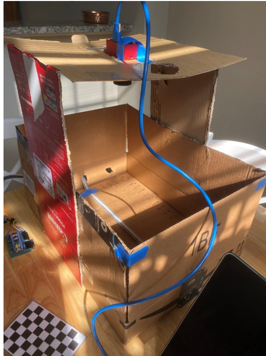
Fig. 1 Setup for LED projectile’s acquisition: lower panel’s dimensions are 11.5 \times 18.5 inches and NVS is 18 inches above LED strip; LED “projectile” propagates left to right across NVS’s field of view (FOV) and is acquired by NVS, connected via USB 3.0 to laptop
