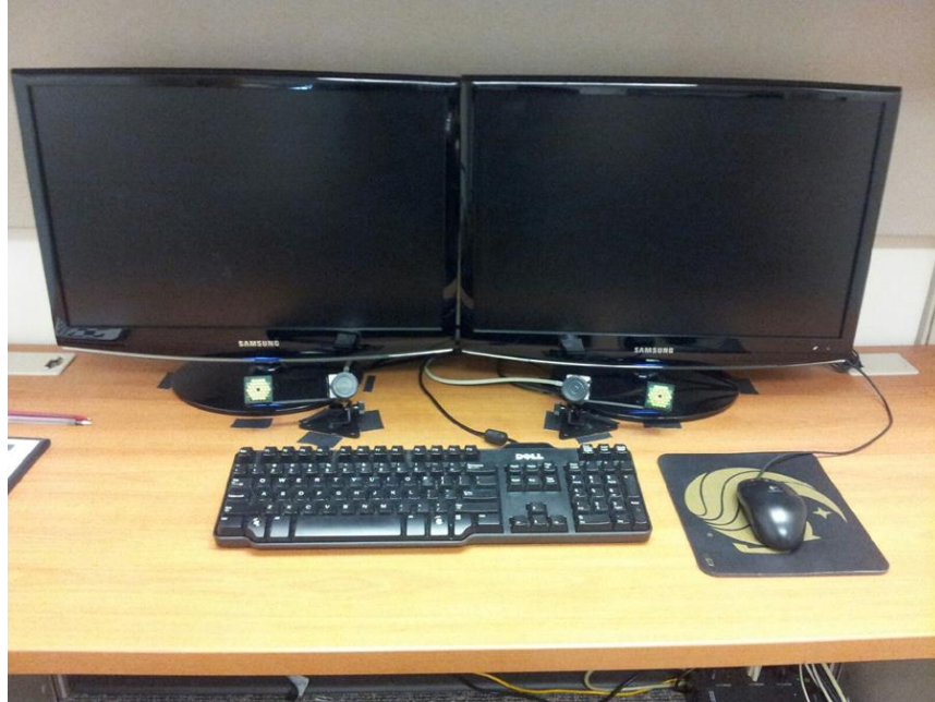
Fig. 3 Experiment station showing the eye-tracking cameras positioned in front of the monitors
