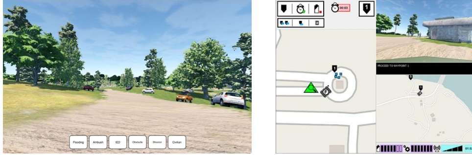
Fig. 2 ASM experimental interface. The left-side monitor displays the lead Soldier's point of view of the task environment. The right-side monitor displays the ASM's communication interface.
