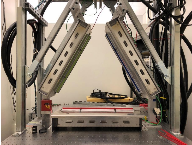
Figure 2. X-ray tubes assembled in the final system geometry assembled on an optical table in the laboratory. The room itself is lead lined, so no covers/x-ray shielding is needed for experiments performed in this space.
