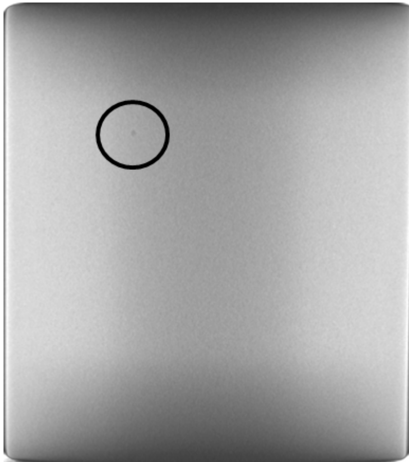
Fig. 4 Front view image of a small void indication (circled) in the interior of the block
