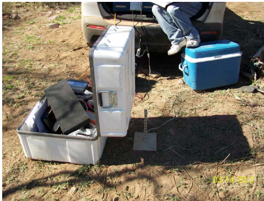
Fig. 11 Sensor deployed for desert environment field demonstration. Placing the sensor where it is shielded from the sun is desirable.
