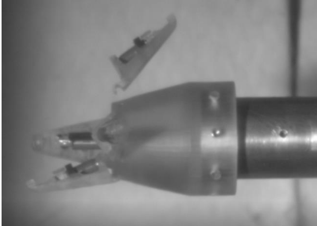
Figure 21 Wind tunnel test of shroud release
