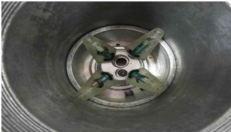
(b) Premature shroud deployment due to adhesive joint failure after test
