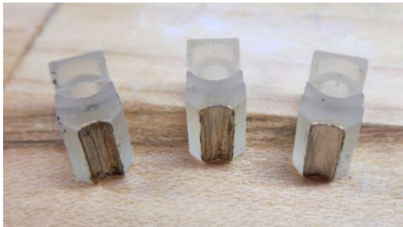
Figure 10 Electrolessly-plated copper on plastic heater finger
