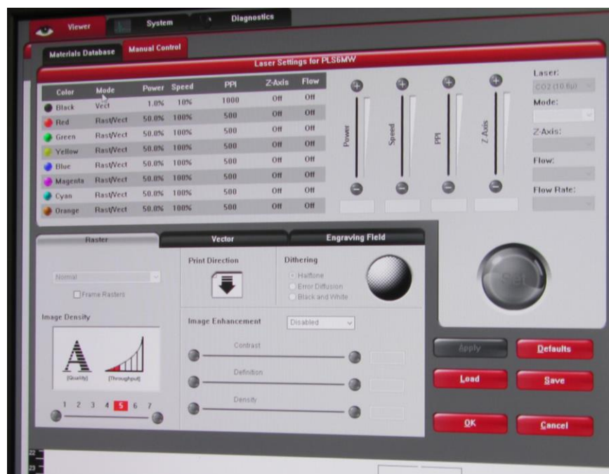
Fig. 9 — Settings in laser engraver software (UCP, ULS). Different speed and power settings are applied to lines of different colors from the imported vector drawing. The settings presented are for sealing (Black) and cutting (Red). Shown above: Black - Vect, 1% Power, 10% Speed, 1000 PPI. Red – RastVect, 50% Power, 100% Speed, 500 PPI.
