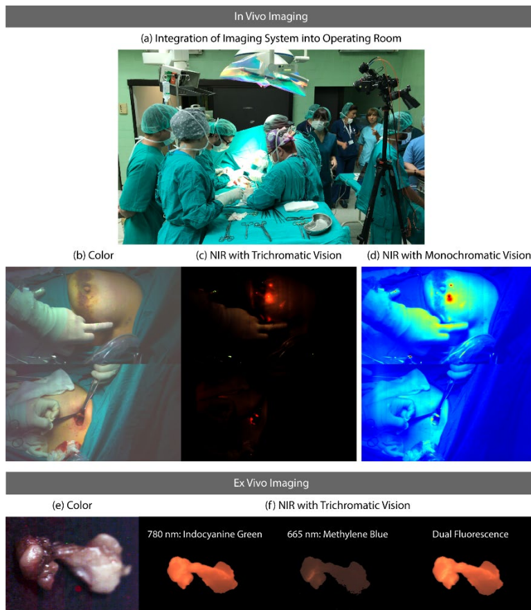
Fig. 5 | Clinical feasibility study with our bio-inspired imaging sensor to map sentinel lymph nodes using indocyanine green and methylene blue. (a) Integration of imaging system into operating room. (b-d) In vivo images before and after the incision for lymph node removal (see also Supplementary Movie S2). (b) Color images. (c) Near-infrared images in trichromatic format (i.e., with spectral discrimination). Injection points and sentinel lymph nodes exhibit high signal-to-background ratio with no false positives due to specular reflections. (d) Near-infrared images in monochromatic format (i.e., without spectral discrimination). Surgical instruments appear as false positives due to strong signal from specular reflection. (e, f) Ex vivo images of a resected lymph node. (e) Color image. (f) Near-infrared image representing indocyanine green alone (left), methylene blue alone (center), and both dyes together (right). Different dyes accumulate in different sites. Abbreviation: near-infrared (NIR).
