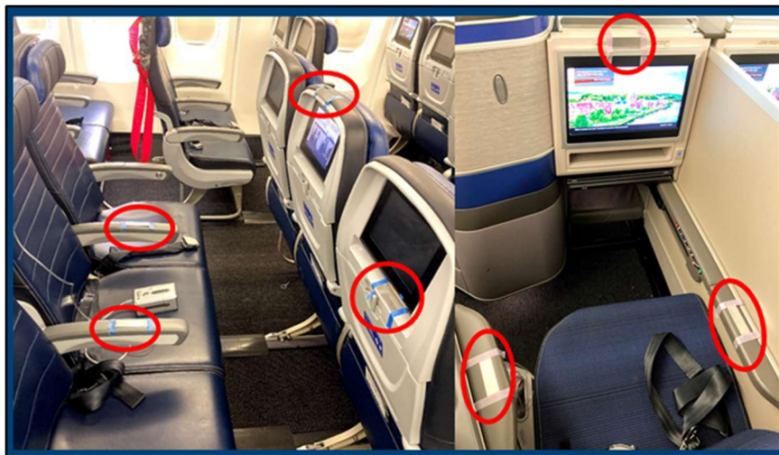
Figure 2. Example coupon locations highlighted in red. Left: Economy seat. Right: First class seat.
