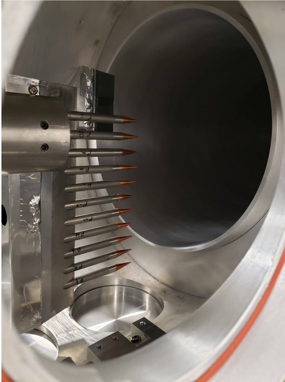
Figure 16: Pitot rake at the Mach 6 nozzle exit to test flow uniformity.
