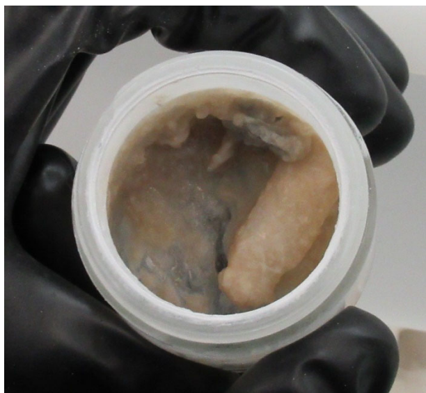
Figure 2. Reaction product of 9 mL DF with \text{H}_2\text{O}+\text{Li}_3\text{N} , after 7 days, sample P19A. The outline of the vial that was used to add water is visible on the right.
