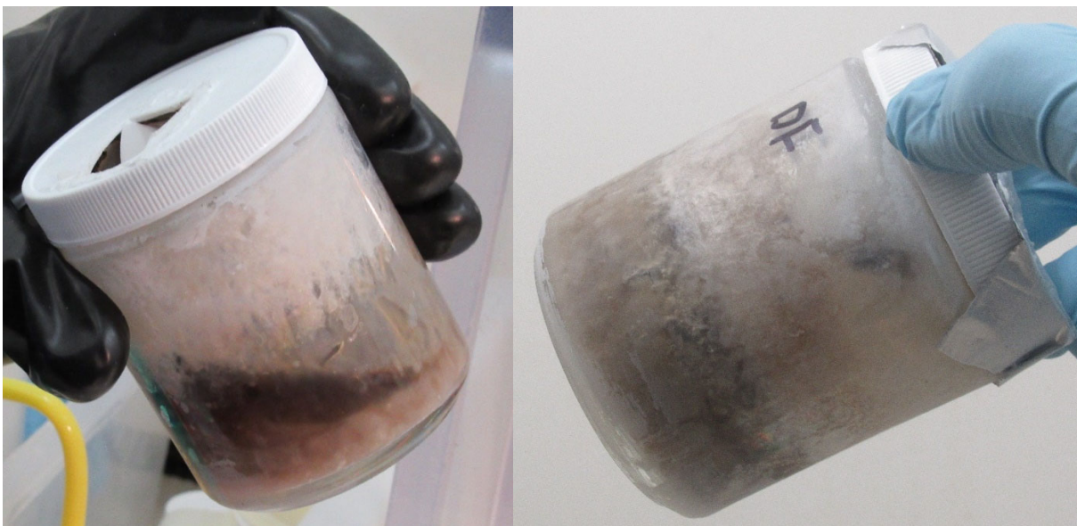
Figure 6. Reaction of 100 mL DF with water and Li 3 N. Left: after 10 days of reaction time (Sample P21A), right: after 2 months. The reaction product is initially a mixed liquid (brownish color) and solid (light brown). DF is not detectable by NMR after <1 day. The lid of the jar couldn't be removed, so a hole was cut in the lid to sample the product. After 2 months, the product is completely solidified.
