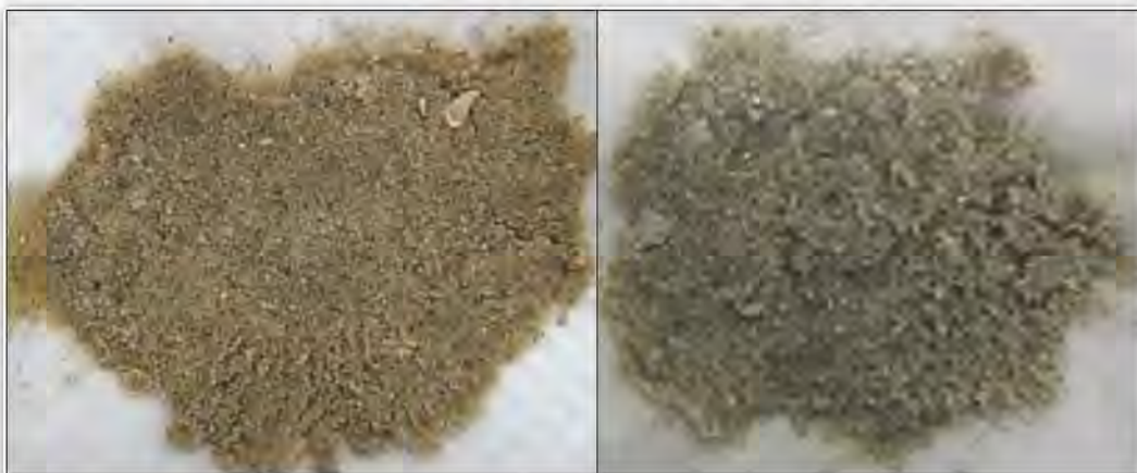
Figure 2-4. The sequential removal of secondary color constituents resulted in a visible change in sediment color from in situ condition (left) dominated by a lightening of the sediments due to an increase in Munsell value and a decrease in the Munsell chroma (right). Color changes remain visible to the human eye, with color shifts resulting in more desirable color characteristics for aesthetics and habitat suitability. Adapted from Berkowitz et al. (2018b, 54).
