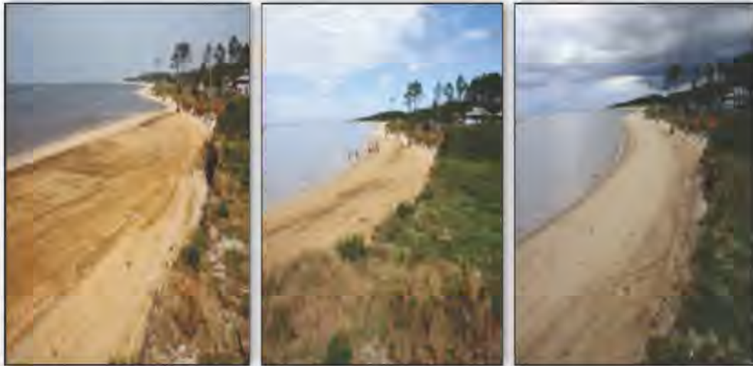
Figure 1-2. Example of dynamic sediment color change following a pilot beach nourishment project near Mobile, Alabama (reproduced from USACE 2013, 71). From left to right, photos represent sediment color immediately following sediment placement, 3.5 weeks post application, and 6.5 weeks postapplication. The sediment color was measured over time, indicating that redder colors transitioned to lighter colors during the monitoring period. However, color changes could not be attributed to any particular mechanism and likely resulted from a combination of mixing with native sand, sediment transport, photochemical bleaching, oxidation, and alteration of iron oxide or other sediment coatings.
