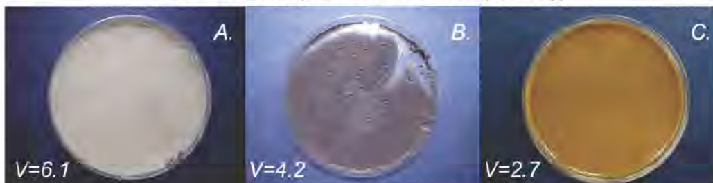
Figure 3-3. Representative sediment samples in the moist state used in the mixing experiment. A is the pure quartz sand (QS); B is the Vicksburg silt (VS); and C is Mississippi River mud (MS). Samples from VS and MS were screened through a 75 \mu m mesh sieve prior to mixing. The initial Munsell value of each sample is indicated in the lower left (6.1, 4.2, and 2.7, respectively).
