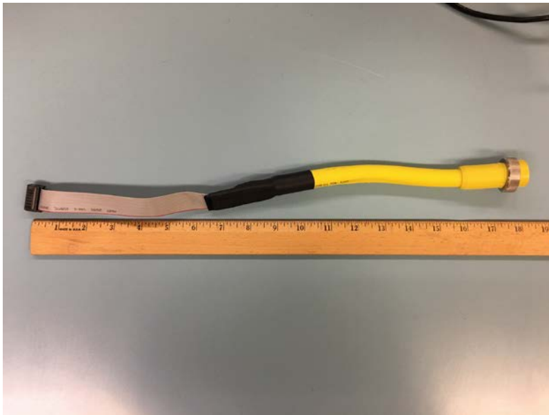
Figure 30. Shorter Cable Designed for Successful Programming of the MS3110 Chip.
