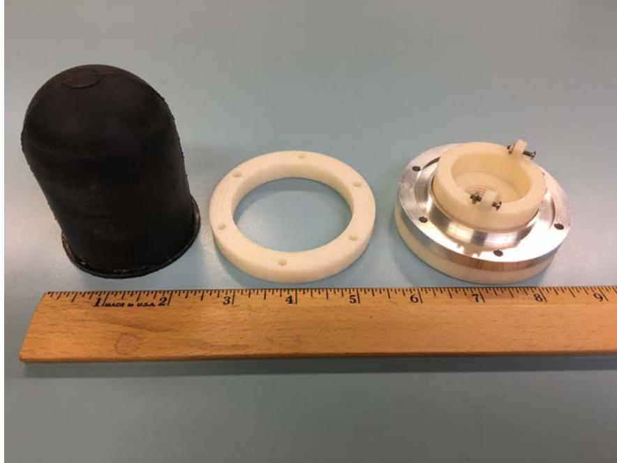
From left to right, the components shown here are (1) the finished Flexane 80 urethane shell, (2) the 3D printed backing ring, and (3) the 3D printed PCB mount and aluminum closure ring.
