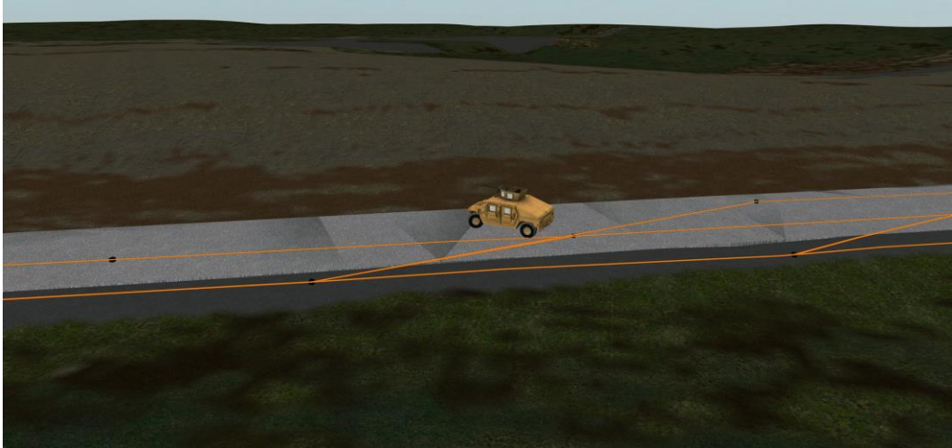
Fig. 8 Vehicle turning in circles while trying to locate the next point on the path. This path movement caused the jagged segments on the scatterplot (see Fig. 4).
