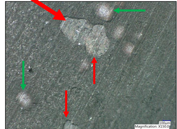
Oxide spallation on MAS crown surface after 50h at 600 °C in engine test
