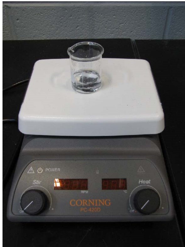
Figure 1: 65°C Hotplate and Beaker for Heating 115, 117 and 1110 Samples to 65°C
