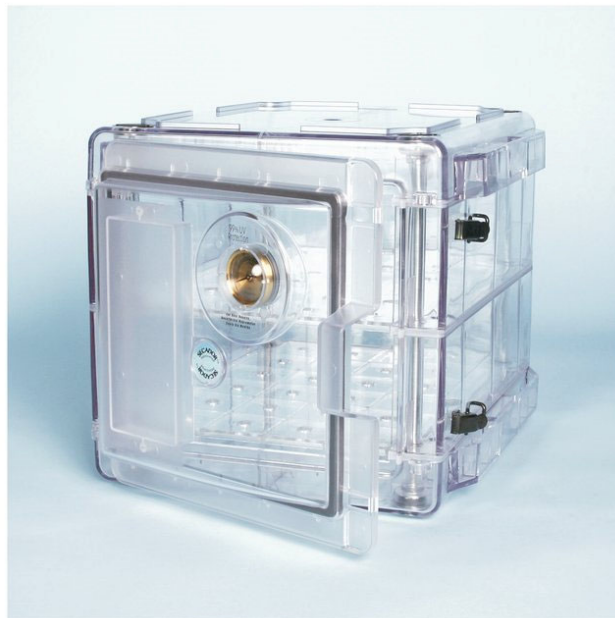
Figure 2: Auto-Desiccator used to Dry and Cool 115, 117 and 1110 Samples
