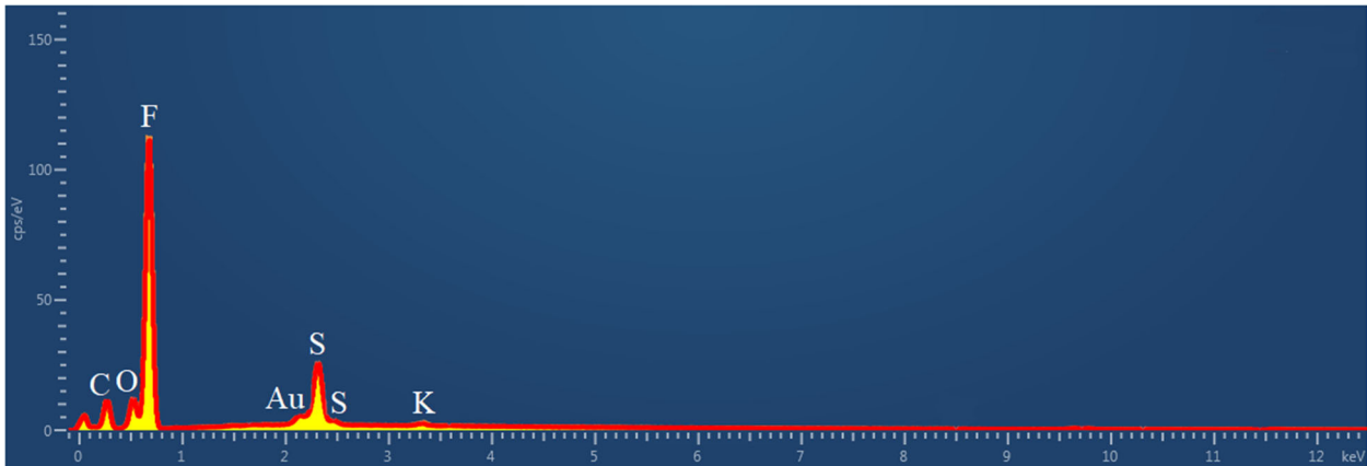
Figure 6: Raw EDS Baseline Measurements of Untested Dry 115, 117 and 1110 Samples
