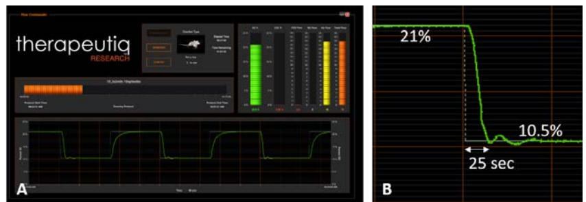
Fig. 1. Front panel of the controller of the Therapeutic hypoxia device (A). We assembled the parts into the functioning device and then got familiar with, tested, and calibrated the device to be able to switch from 21% to 10.5% (i.e., 50% oxygen level) within 20-30 sec (B).
