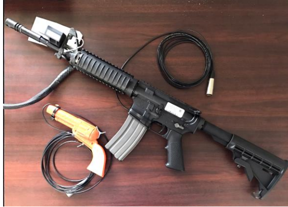
Figure 16. Custom hardware installed on a cap gun (used in another part of this study, results not discussed here), and carbine simulator (from the EST2000 system) used during the SH/SP tasks.
