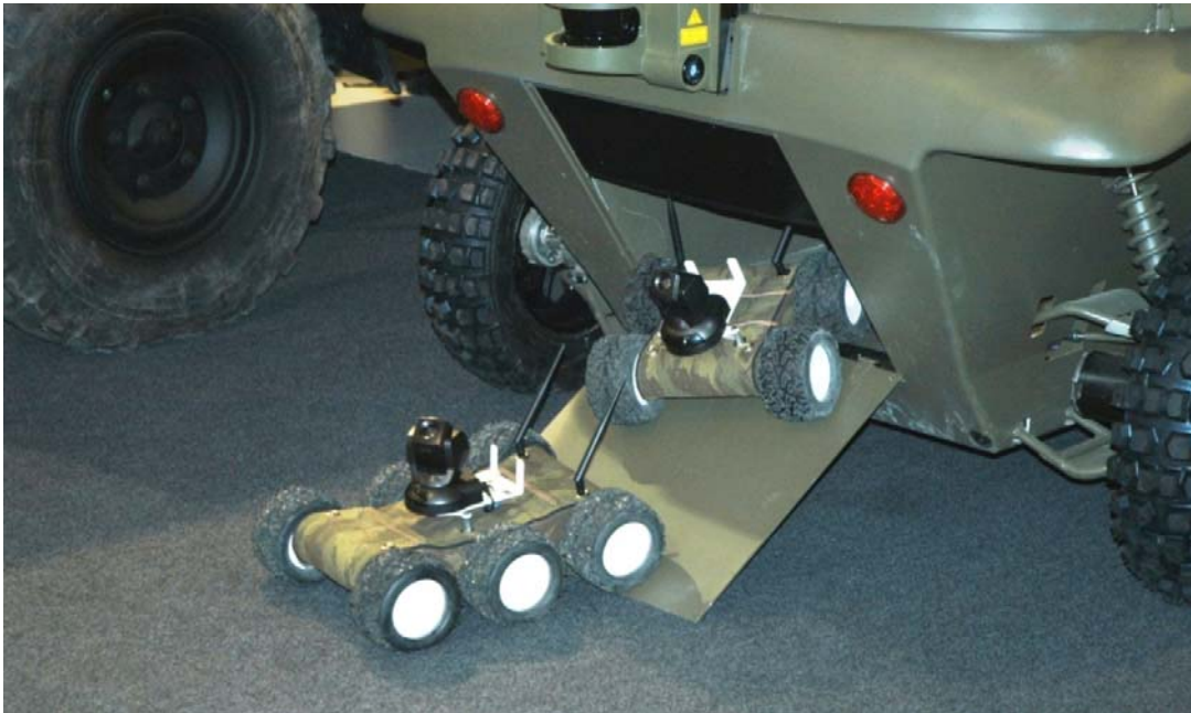
Figure 65. France's Thales Trooper R Unmanned Ground Vehicle Disgorgeing Smaller UGVs on Display at Eurosatory 2008
