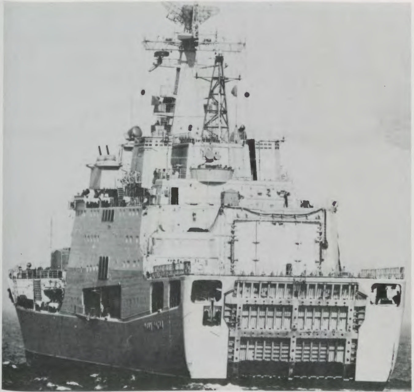
Defense production includes the new IVAN ROGOV-Class amphibious assault ship. Judging by IVAN ROGOV's characteristics, the ship can carry three air-cushion landing craft, a Naval Infantry Battalion, armored personnel carriers, tanks and helicopters.
