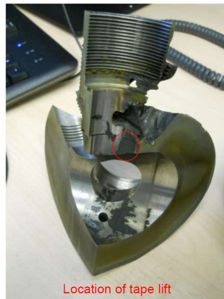
Figure 4. The sampling location of the metal deposit which was found to contain ~10% elemental titanium.
