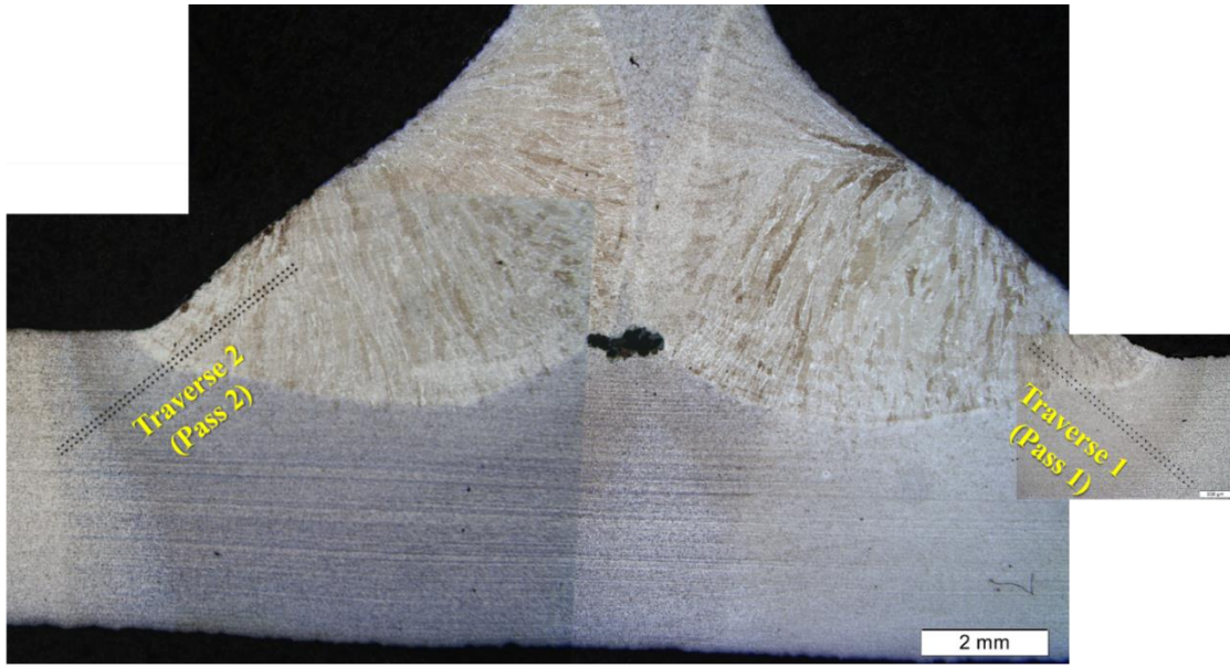
Figure 19. Composite image of light optical micrographs of the HSLA-65 fillet weld showing placement of microhardness indents. Indents appear as parallel lines of black dots on the left and right sides of the image.
