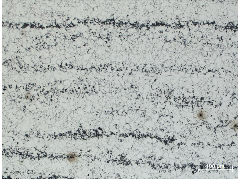
Figure 65. Representative microstructure from the HSLA-65 dilatometry specimen heated to a peak temperature of 825 °C (1517 °F) and continuously cooled at 1 °C/s (1.8 °F/s). Banding of pearlite (dark etched constituent) is apparent at low magnifications.
