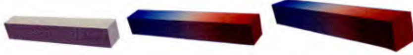
Figure 19: Reconstructed deformation from data on a soft polymer showing the reference (left), first deformed (middle) and ninth deformed (right) configurations. VSI discovers deformation mechanisms from these data.
