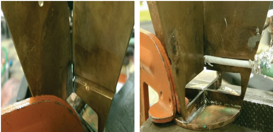
Figure 56. (a)Feed slot milled on the fin side (b) Inserted coax which turns into a probe and feeds the ridge.
