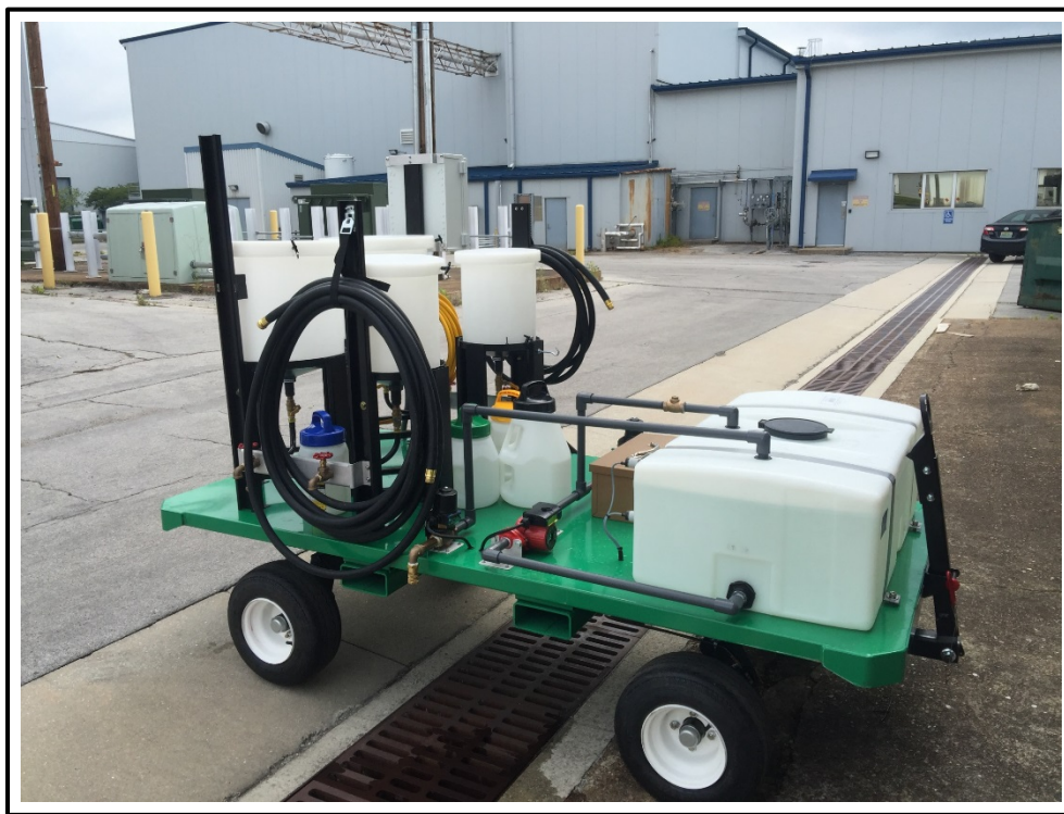
Figure A-3. Liquid delivery system.
