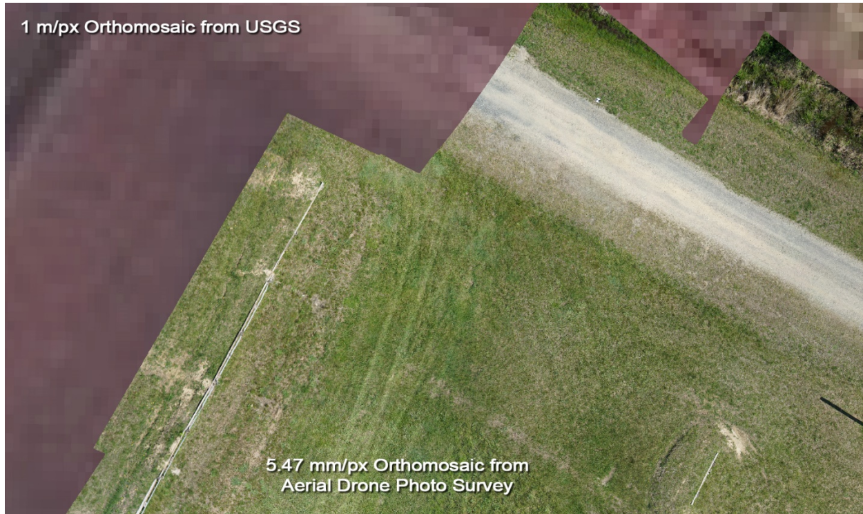
Figure 33. Comparison of aerial drone survey vs. orthomosaic available from United States Geological Survey (USGS)
