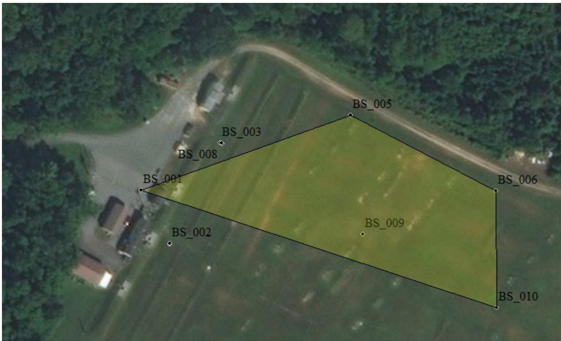
Figure 4. Base station locations used for the most accurate correlation, shown as vertices
