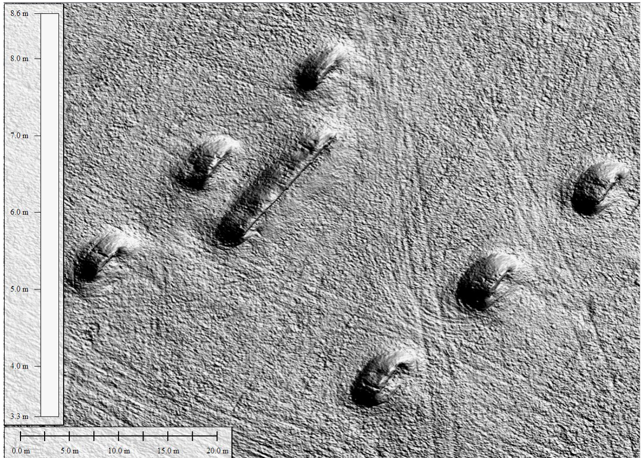
Figure 29. Close-up showing detail of DSM created from aerial photogrammetry
