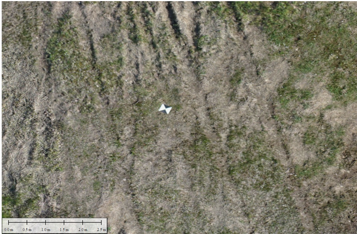
Figure 31. Example GCP captured from quadcopter
