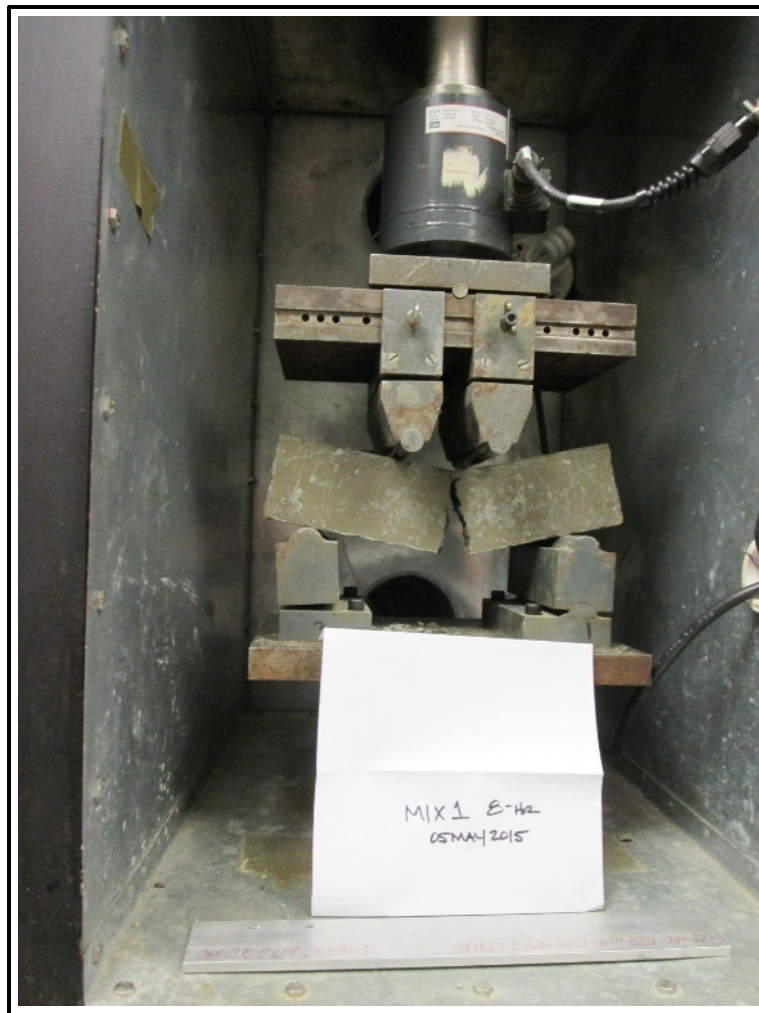
Figure 3-8. Mix 1 Baseline flexural at 8-hr test age in the testing apparatus.
