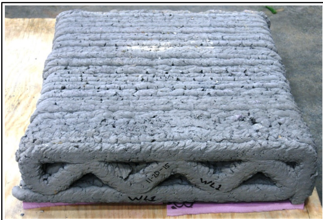
Figure 5-7. Printed wall section for BLS testing.
