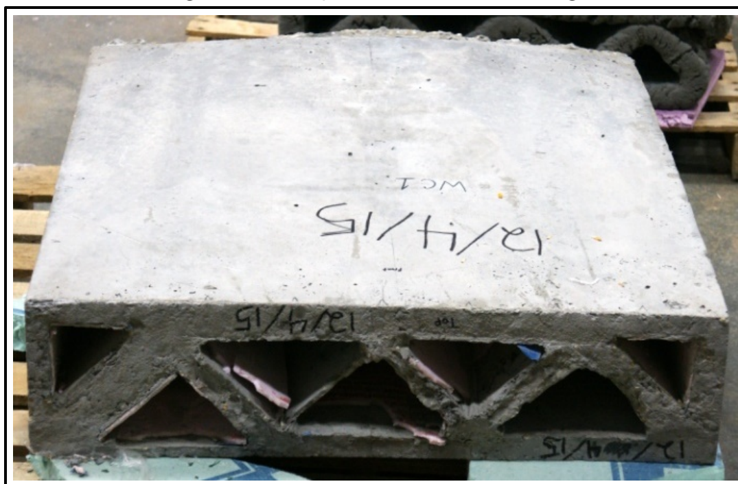
Figure 5-8. Cast-in-place wall section for BLS testing.
