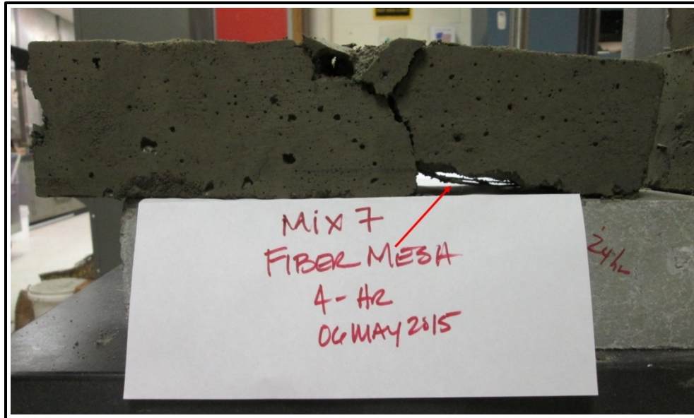
Figure 3-10. Test beam for 4-hr Baseline mix with aramid fiber mesh reinforcement.
