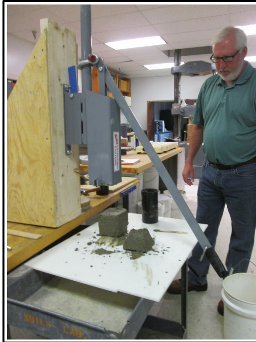
Figure 3-3. Clogged material removed from extruder.
