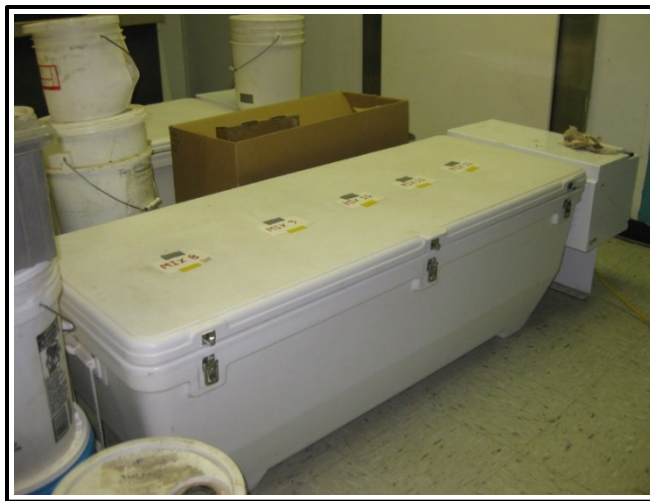
Figure 3-14. Curing box used in the laboratory testing to supply a moist curing environment.
