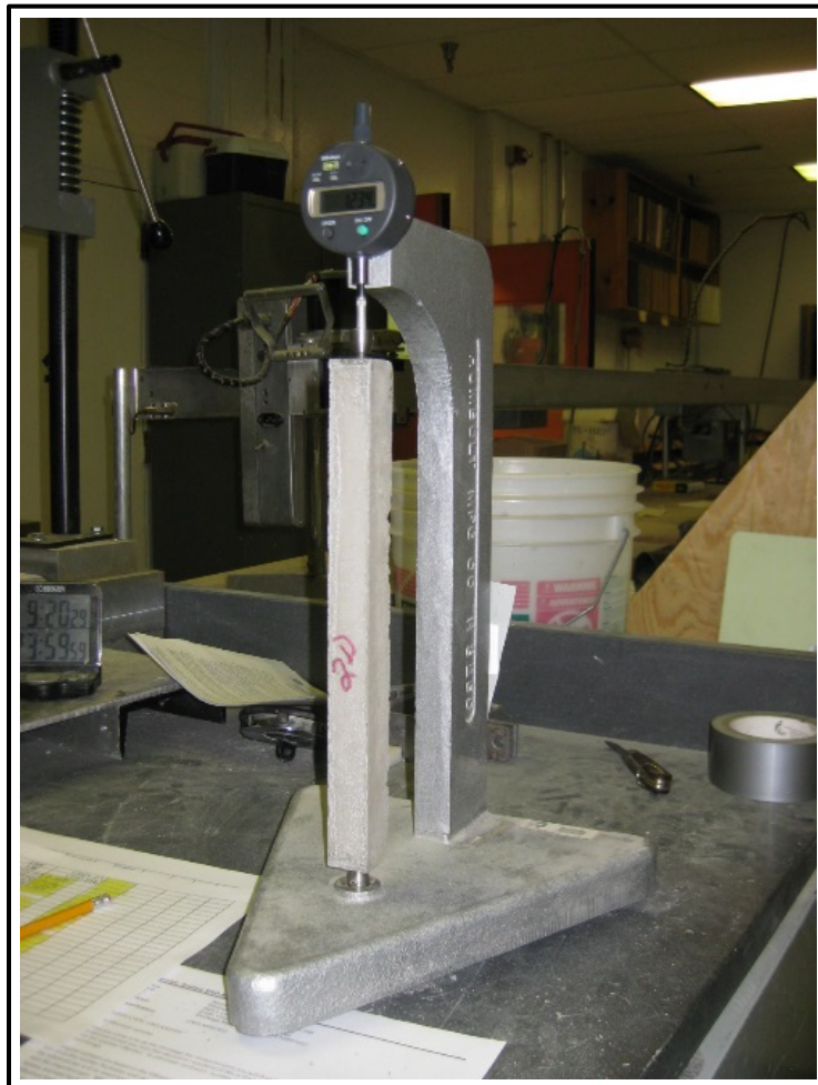
Figure 3-17. Length comparator apparatus with digital readout.
