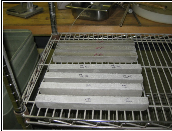
Figure 3-16. Test specimens were placed on wire shelving to continue air storage.
