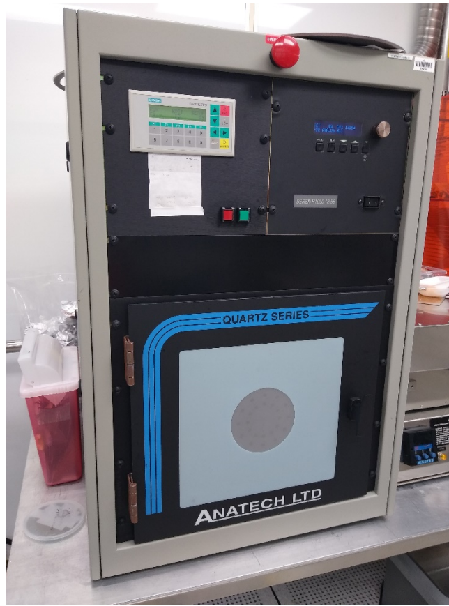
Fig. 11 Anatech SCE1000 Barrel Asher
