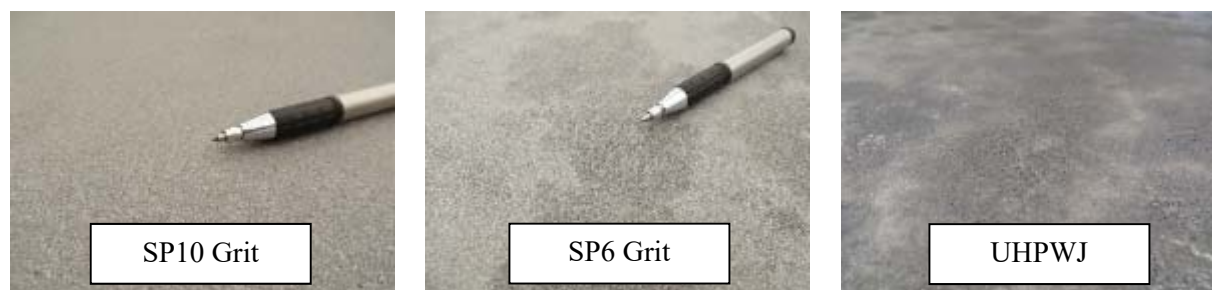
Figure 7 – Close-up images of each surface condition on the DDG missile deck
