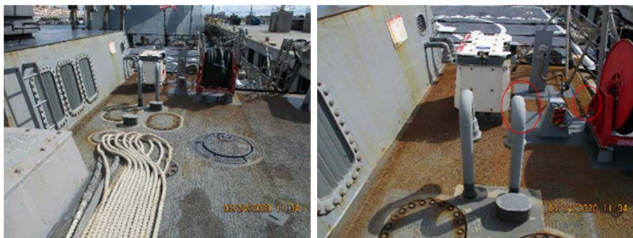
Figure 41 – Close-ups of section 1 that received 100% SP10 Grit surface preparation of the deck and appendages
