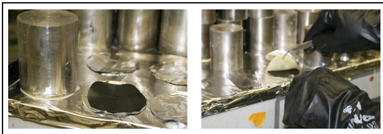
Figure 5. Contact sampling setup. The image on the left shows an in progress sample (left) and a contaminated butyl coupon about to be treated with a latex sampler. The image on the right shows the latex sampler being removed from the rubber coupon following the 15 min touch.
