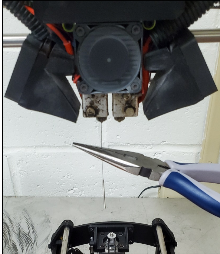
Fig. 15 Nozzle cleaning with needle
