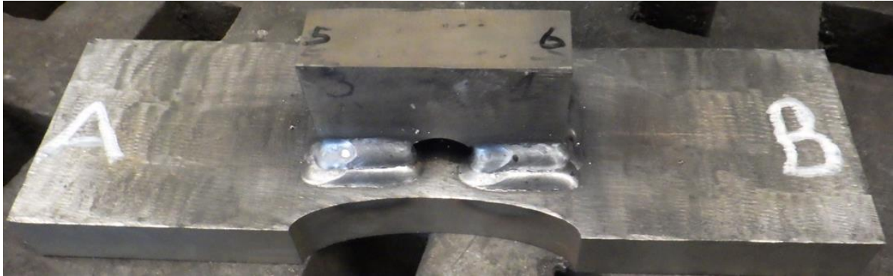
Figure 3. Post-welding to produce the final component, Specimen #3.
