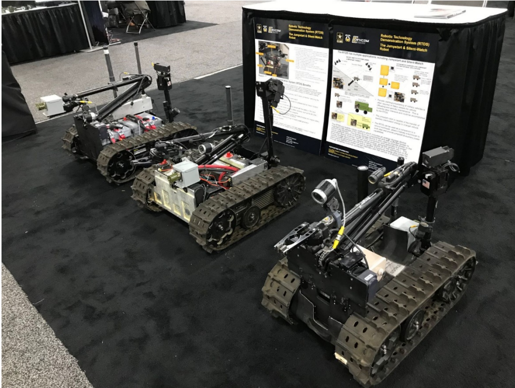
Figure 11: Single 6T, Dual 6T, and Hybrid Fuel Cell 6T TALONS (multiple NATO receptacle configurations shown)
