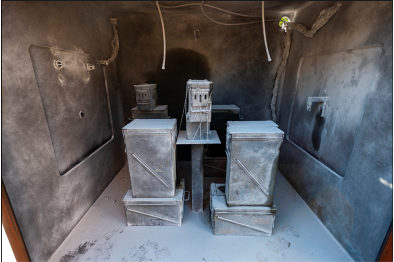
Figure 2: Opened 148 ft 3 test chamber with clutter (ammo cans added to create obstructions)
