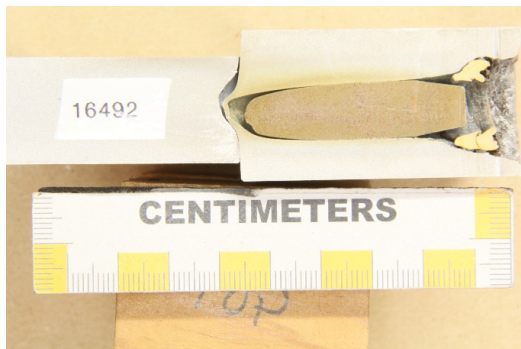
Left: Cross section of 12.7-mm APM2 penetrator
