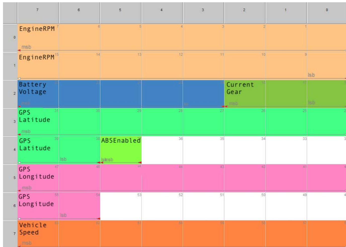
64-bit CAN data field description defined in DBC: CAN signals (color), unused bits (white)
