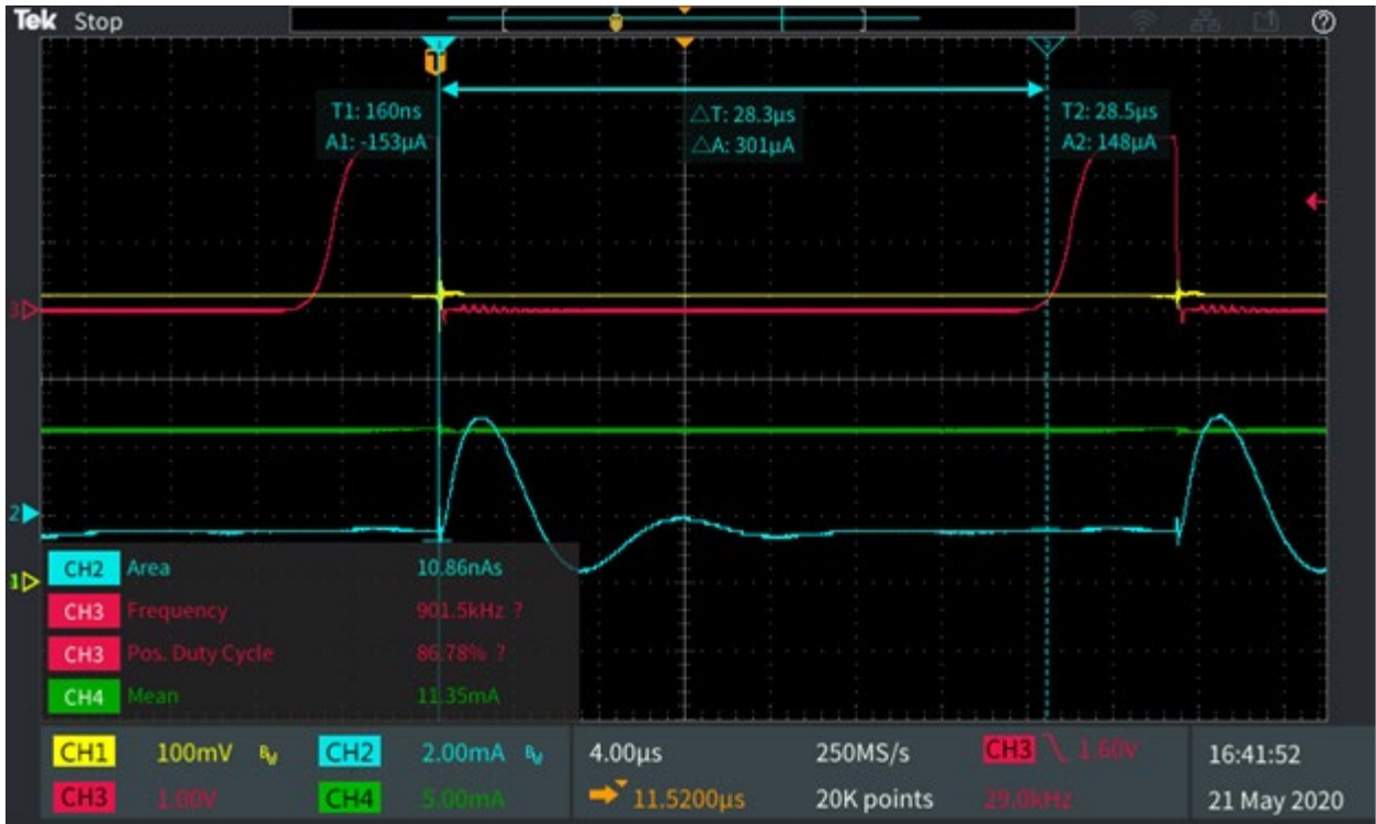
Figure 23. R_{mfc} = 32 \text{ ohm} , Current to battery goes to zero before next PWM.
