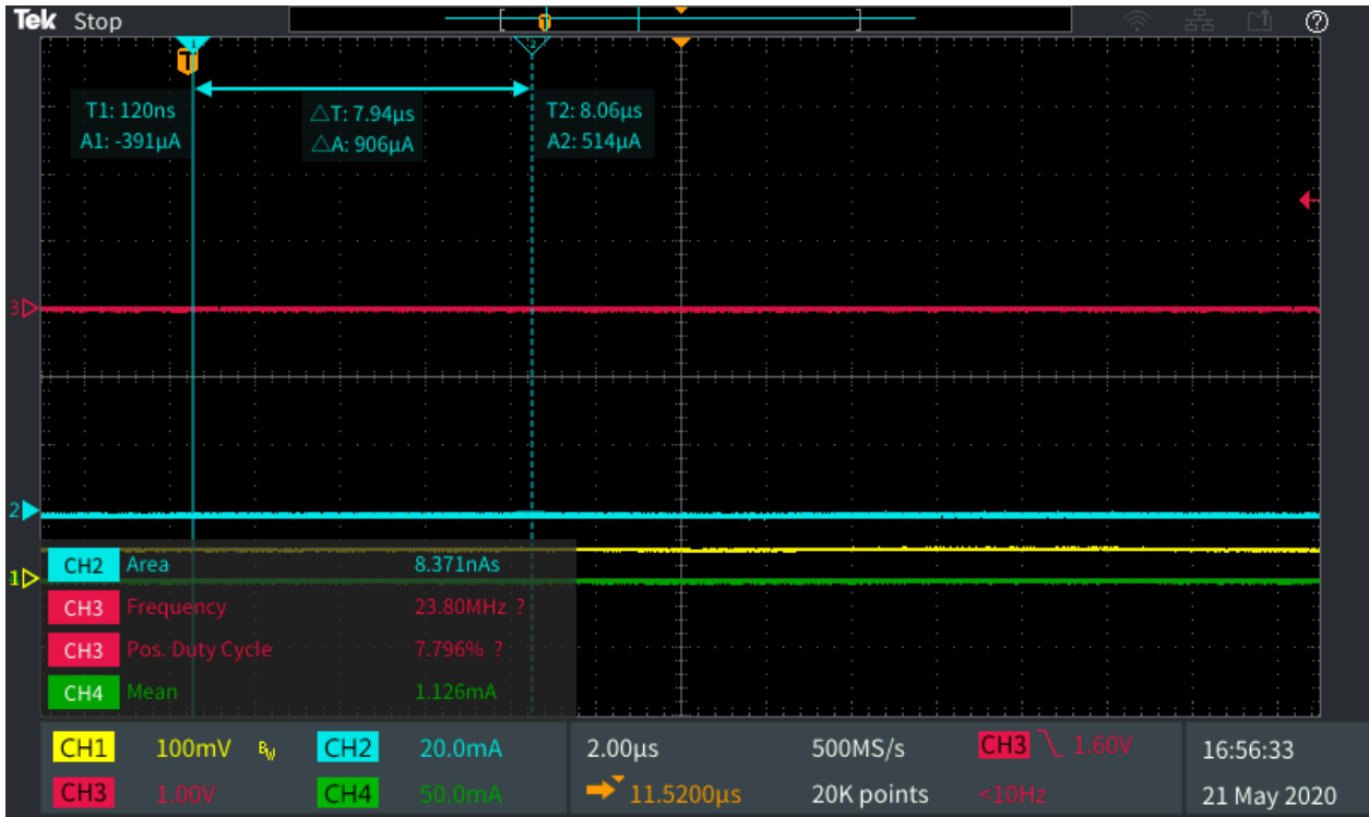
Figure 22. Offsets with MFC supply off for R_{mfc} = 1 \text{ ohm} .
