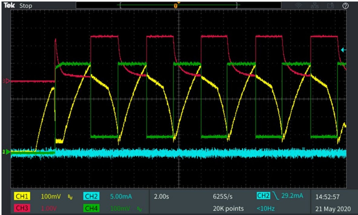
Figure 26. Start-up issue due to low power MFC causing start stop cycle. R_{mfc} = 210 ohms, Yellow MFC voltage, Blue MFC current, Green Pmos gate voltage, and Red VDD_PWM.
