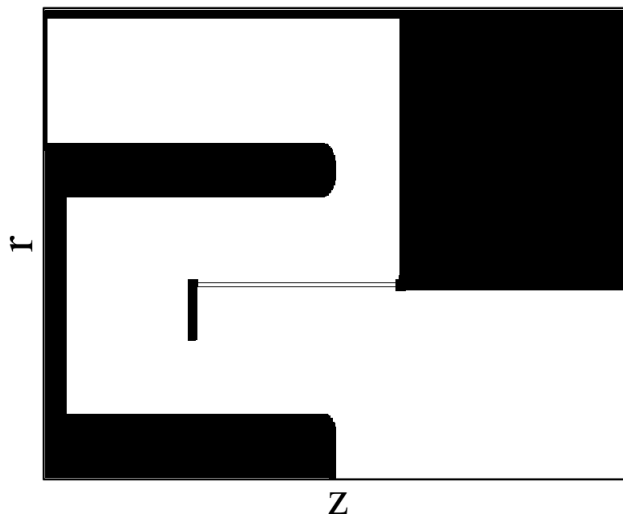
Fig. 9: Modified geometry of coaxial vircator with rounded cathode, reduced inner cathode radius, and smaller reflecting ring.
