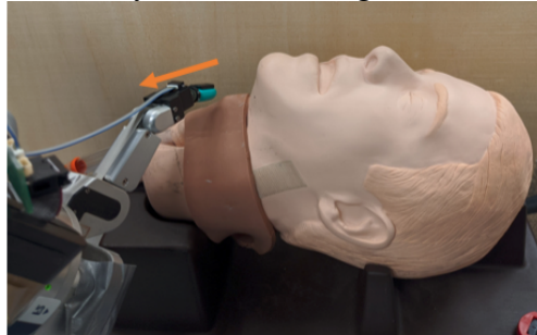
Figure 33: The robot performing palpation surgery with high-fidelity Syntouch probe.
