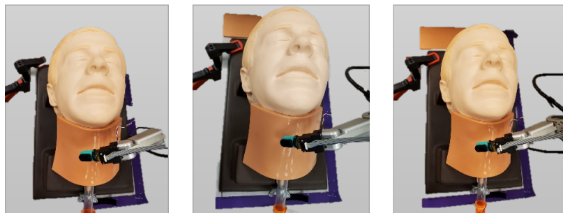
Figure 34: Skins of different thickness for robot to learn a generalized feature registration.
