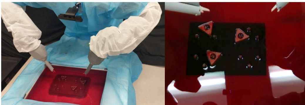
Figure 8. The system with the blood peg transfer setup and the view from the robot camera.
