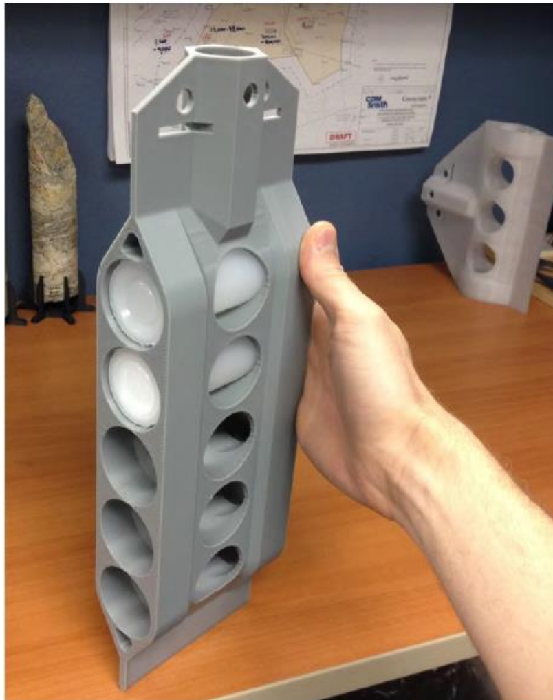
Figure 23 Prototype sampler frame to deploy cylindrical samplers to assess metal contamination in sediments.
