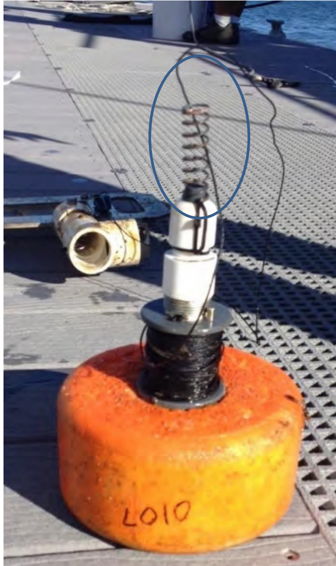
Figure 11 A spring attachment design (circled) that interfered with the line spool release and was abandoned.
