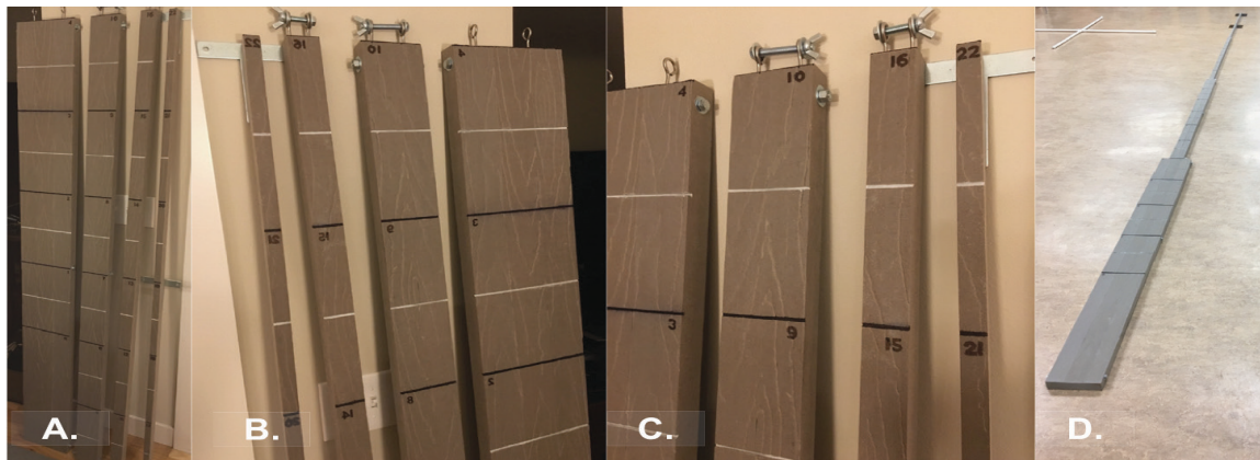
Figure 2. Design and construction of our Narrowing Beam Walking Test (NBWT). (A) View of the entire length of each segment with corresponding distance marks etched in. (B and C) Zoomed in views of each segment, highlighting the bolt & eyehook distal fixtures used to connect adjoining beam segments. (D) View of the NBWT with each segment connected and ready for testing.
