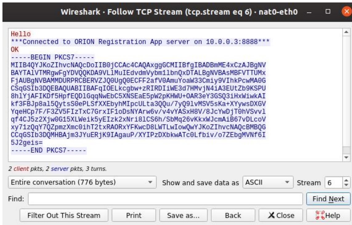
Figure 5.1. Wireshark Capture of Application TCP Stream
